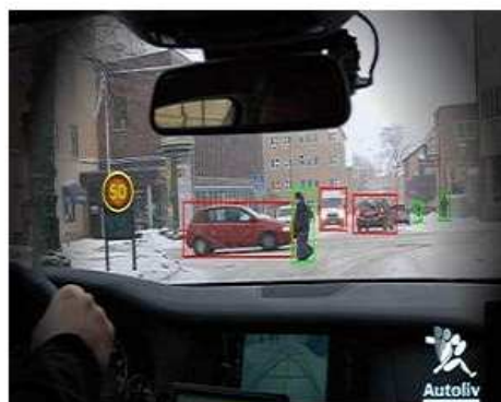
Figure 21. Forward object detection using camera
