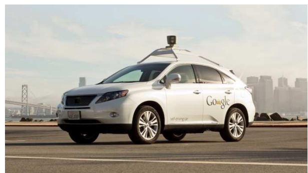
Figure 17. Google's self-driving car with LIDAR on roof
