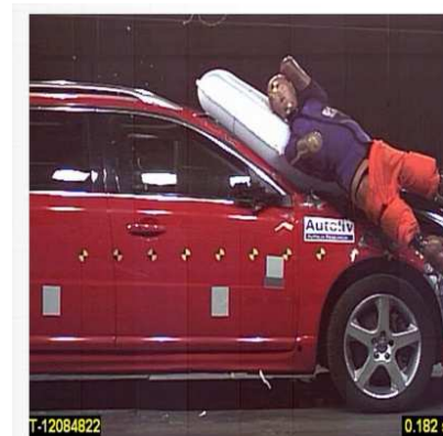
Figure 33. Pedestrian protection 2: Pedestrian airbag
