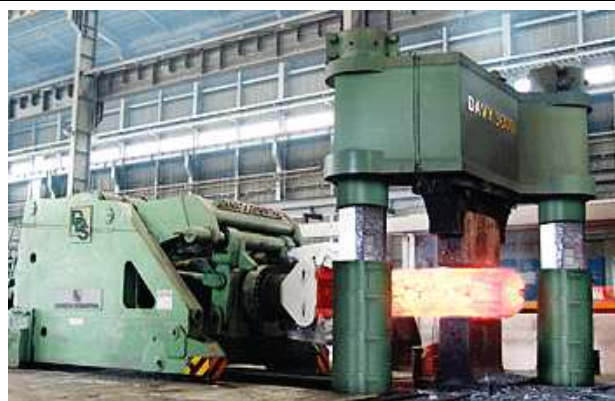
Figure 12. Press used to turn raw materials into a round shape
